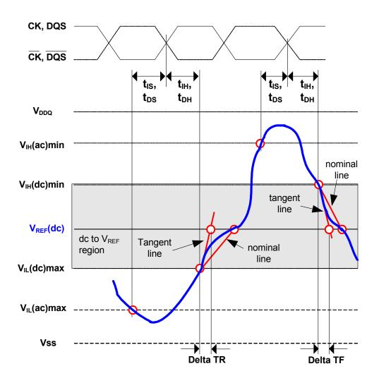
$\frac{\text{Hold Slew Rate}}{\text{Rising Signal}} = \frac{\frac{\text{Tangent line[VREF(dc)-V_{IL}(ac)max]}}{\text{Delta TR}}}{\frac{\text{Hold Slew Rate}}{\text{Falling Signal}}} = \frac{\frac{\text{Tangent line[V_{IH}(ac)min-VREF(dc)]}}{\text{Delta TF}}}{\frac{\text{Delta TF}}{\text{Delta TF}}}$
