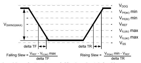
edges and the range from  $V_{\text{REF}}$  to  $V_{\text{IL}(ac)}$  max for falling edges as shown in the figure below.
