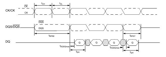
Figure -- Data output (read) timing
