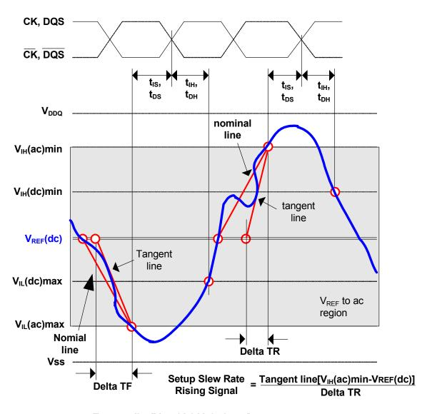
Setup Slew Rate Falling Signal = Tangent line[VREF(dc)-V<sub>IL</sub>(ac)max]
