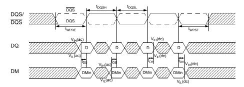
Figure -- Data input (write) timing
